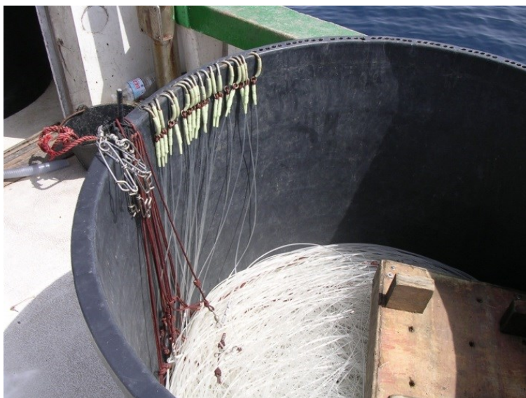
Figure 44. Typical basket, where the mainline is stored.
