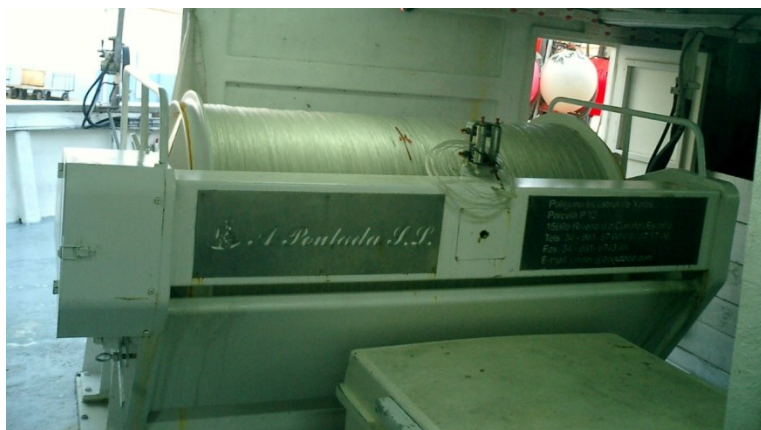
Figure 45. Hydraulic reel, where the mainline is stored.
